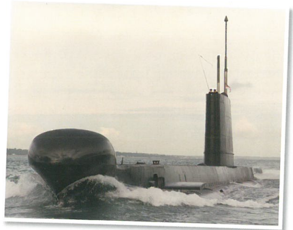
HMS Otter, conventional submarine with diesel/electric drive showing ballast tanks along the sides of the submarine. You can see four of the main vents just above the waterline on the port side. The large dome houses the main sonar array.
